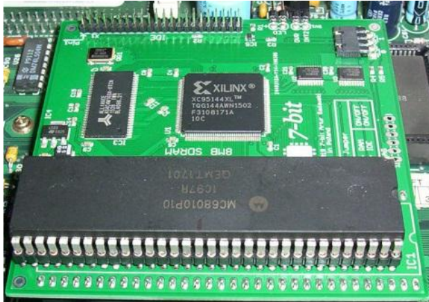
Correctly installed MC68000 chip
