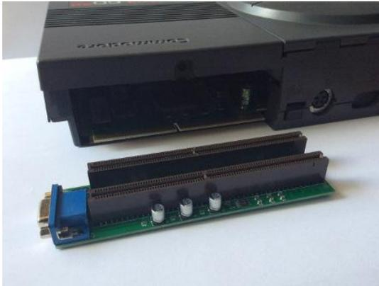
Next, Wicher CD32 card should be installed into the CN1 port of the CD32 Expansion Slot.
