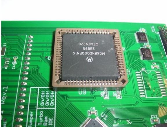
Correctly installed MC68000 chip
