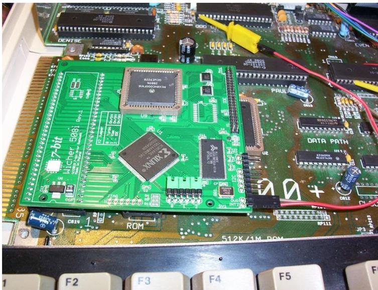
As the next step, one should connect the two provided cables to the card's SV1 port, following the instructions presented below.
