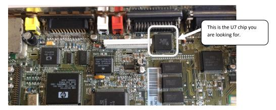
Next you should place Sum adapter's socket on the U7 chip and push it gently in order to make it appropriately attached to the chip.
