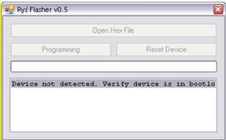
When application detects connected Ryś adapter it will enable **Open Hex File** button. Firmware update procedure looks as follows:
