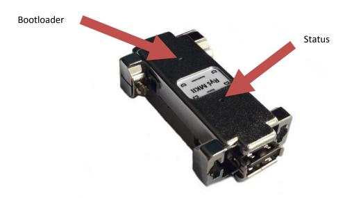
When pressing and holding the **Bootloader** button, one should connect the device via USB A-A cable to the PC running Windows. After being recognized by Windows OS, adapter switches into **Bootloader** mode which is confirmed with continuous pulsation of the **Status** LED.
